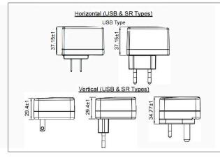
Case Size: Horizontal: USB: 55.6L x 27.1W x 37.15H (mm) SR: 55L x 25W x 36.7H (mm) Vertical: USA, EU: 53.46L x 41W x 29.4H (mm) UK: 53.46L x 41 W x 34. 77H (mm) AC Plug: (K) UK Pin (U) USA Pin (E) EU Pin Weight: 70g
