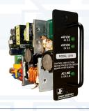
Jasper Electronics Model TC2219 component power supply module is fully compliant to the Advanced Transportation Controller (ATC) Cabinet Standard 5301, v02.02, March 18, 2019, and designated as ATC 5301 Model 2219. Generally, Model TC2219 is a 2-output switching power supply capable delivering up to 120 Watts DC and intended specifically for use in ATC High Voltage (HV) Cabinets. These are
