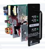
TC2217 ATC power supply module is fully compliant to the Advanced Transportation Controller (ATC) Cabinet Standard 5301, v02.02, March 18, 2019, and designated as ATC 5301 Model 2217. Generally, Model TC2217 is a 2-output switching power supply capable delivering up to 120 Watts DC and intended specifically for use in ATC High Voltage (HV) Cabinets. These are designed for non-redundant "cold pluggable" installation in the end product.
