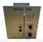
TC206L is a switching power supply delivering up to 120 Watts of DC power through a single, regulated +24V DC output. It provides full output regulation across changes in AC Line voltage and output load over the full operating temperature range of -34°C to +74°C. Power Factor Correction is provided. This model has a functional AC input range of 80V AC to 270V AC input and 47 to 63Hz. 206L is an open frame design, with the
