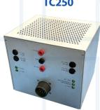
TC250 NEMA Power Supply module designed to meet or exceed the requirements of NEMATS 2-2016 V03.07, as required for TS-2 Type 1 and TS-2 Type 2 traffic control cabinets that incorporate Bus Interface Units. This unit is rack mounted and fully enclosed, providing up to 132 Watts to two regulated DC outputs and a single unregulated AC output, and include a line frequency reference for use in detector racks, load switches and auxiliary components of traffic control cabinets.
